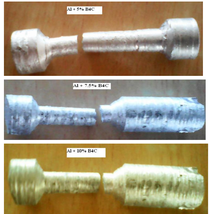
Figure 7: Tensile Test on various Al-B 4 C Compositions
