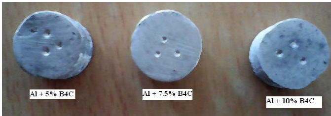
Figure 8: Brinell Hardness Test on various Al-B 4 C Compositions
