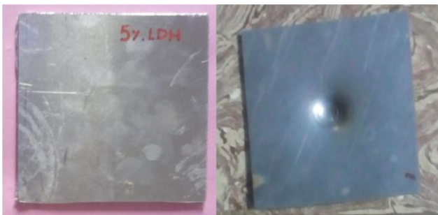
Fig 4.8 Ericission cupping test specimen before and after testing
