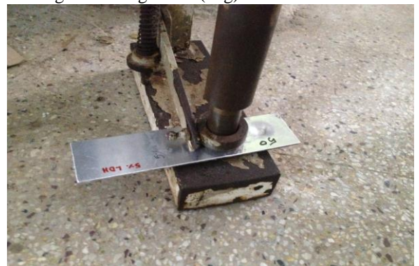
Fig 4.5 impact resistance test setup.
