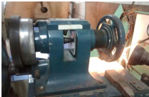
Fig 4.7 Ericission cupping test setup
