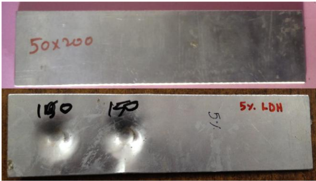
Fig 4.6 Impact resistance specimens before and after testing
