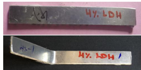
FIG. 4.4: Flexural test specimens before and after testing
