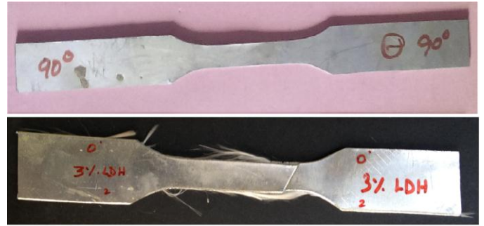
Fig. 4.3: Tensile test specimens before and after testing
