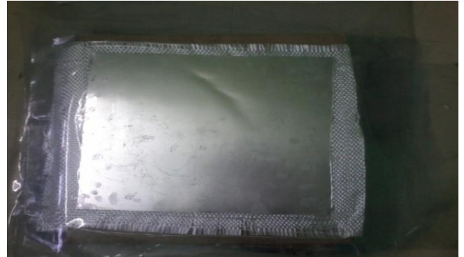
Fig 3.1: Covering of aluminum sandwich sheets with plastic cover
