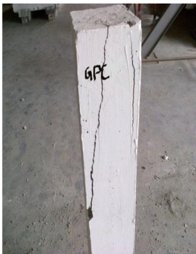
Fig 9 GPC column after testing
