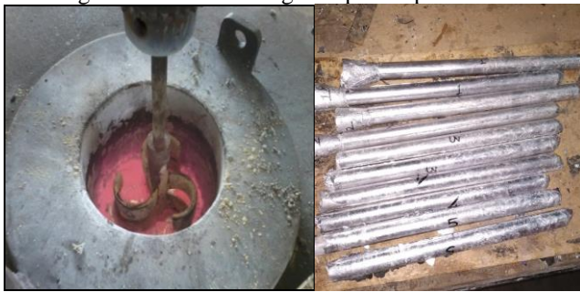
Fig. 1 Stir casting set up and specimen
