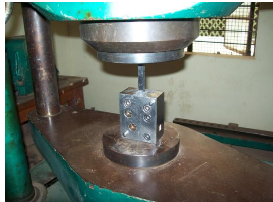
Fig 2. Schematic showing the assembled view on UTM ready for load to be applied
