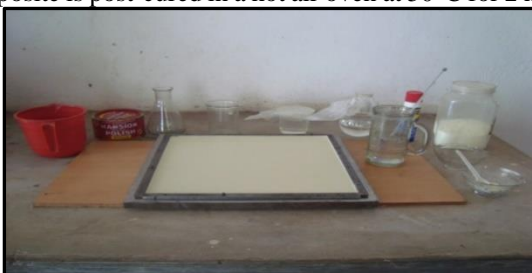
Figure 2: Open Mould Cavity
