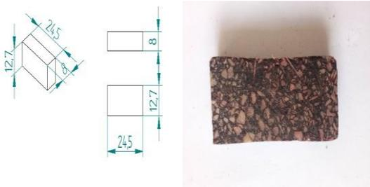
Fig 3. Compression test prepared specimen
