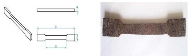
Fig 2: Tensile test prepared specimen
