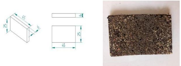
Fig 7. Water absorption test prepared specimen
