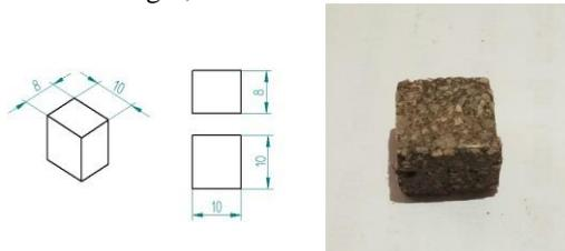
Fig 5. Hardness test prepared Specimen Size
