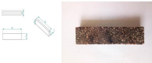
Fig 4. Flexural test prepared specimen
