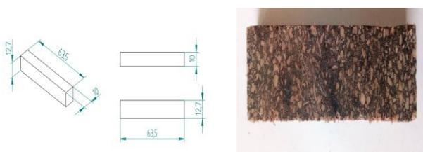
Fig 6. Impact test prepared specimen
