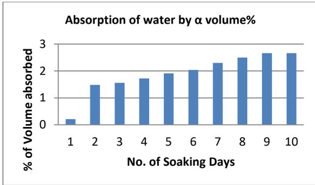
Fig. 11: Effect of treated fibers and filler contents with PF resin on the water absorption test specimens of natural composites
