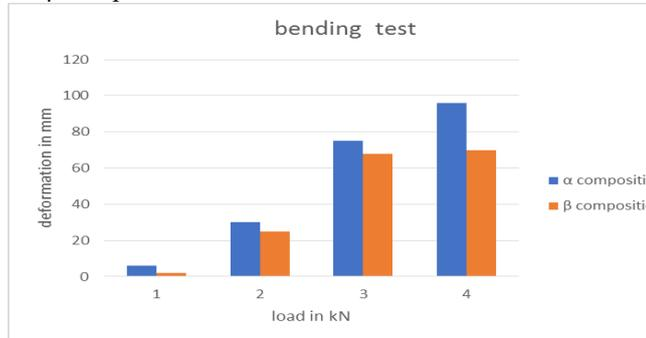
Fig. 9. Effect of treated fibers and filler contents with PF resin on the bending strength specimens of natural composites.
