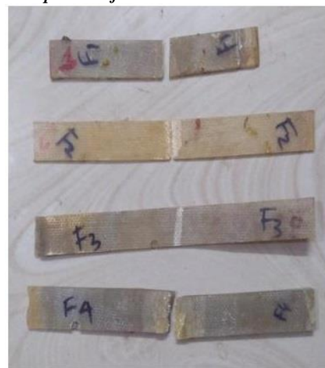
Fig.4 Flexural Test using UTM
