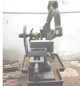
Fig: 3.2 Samples were machined by Using Power Hacksaw
