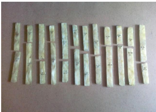
Ø Shows the Fabricated & Tested of Composite Specimens
