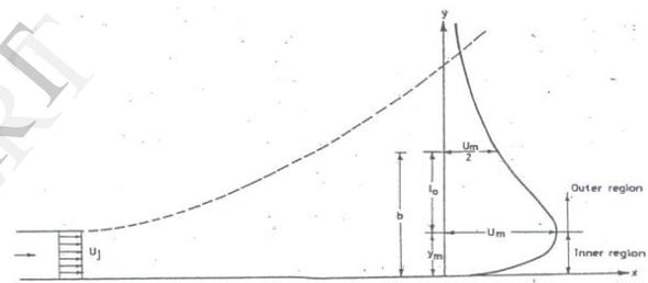
Fig.1 Definition sketch of a wall jet
