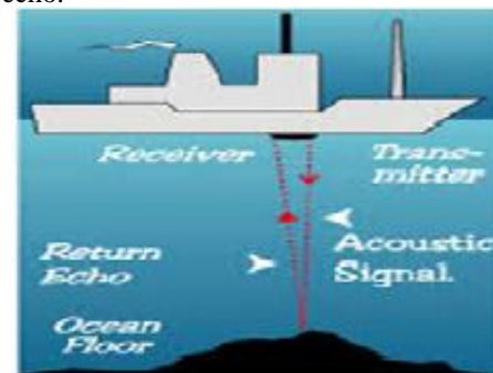
Fig. 1. Ultrasonic transducer transmitting acoustic signal and receiving corresponding reflected echo from the sea bed
