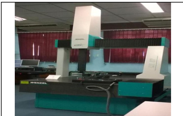
Fig.2: Wenzel \mu Star CMM [Courtesy: Metrology Group, APMF, CSIR-NAL]
