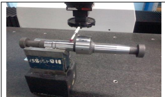
Fig. 1: The cylindrical component/ part during data points collection
