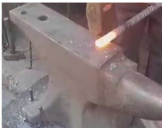
Figure 3: Forging process for diagonal bars.
