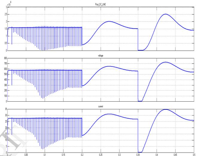
Figure 8. The Power, Voltage And Load Current For The Second Case
