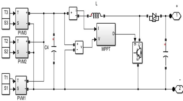
Figure 3 circuit diagram and topology control photovoltaic system
