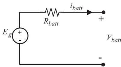
Figure 4: Equivalent circuit for the battery
