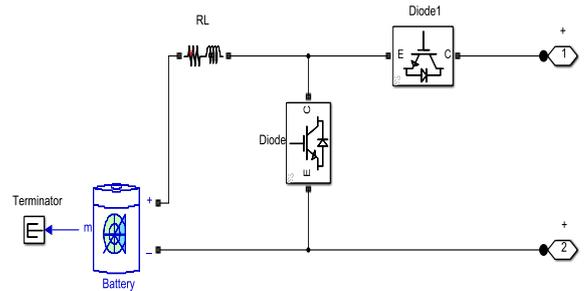
Figure 5: The circuit diagram of a battery storage system
