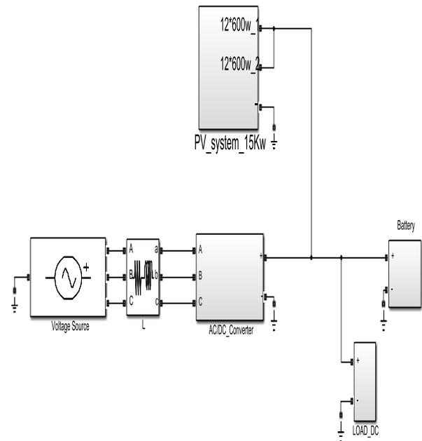
Figure 1. Schematic diagram of DC micro-grid simulations
