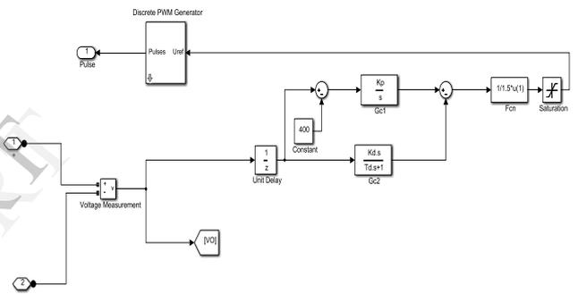
Figure 6. Block diagram of the proposed control battery storage system
