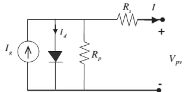
Figure 2: Equivalent circuit of a photovoltaic array
