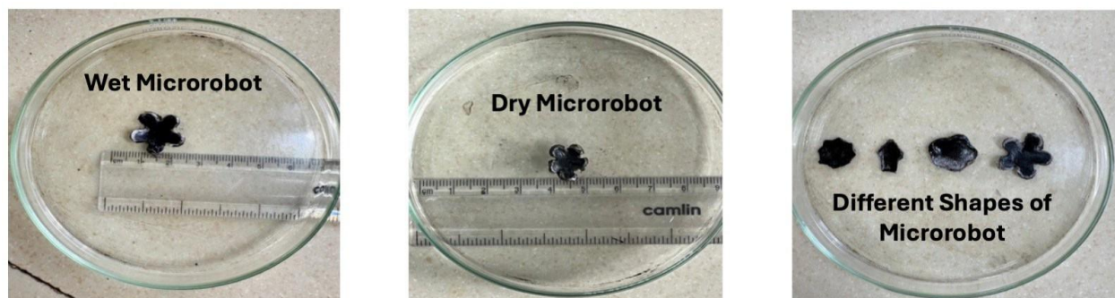
Figure No. 4.6: Measurement of Wet and Dry Microrobot and Different shapes of Microrobot
