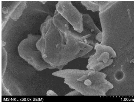
Fig. 2: SEM photograph of \text{CaAl}_2\text{O}_4: \text{Eu}^{2+}, \text{Nd}^{3+}, \text{Gd}^{3+}
