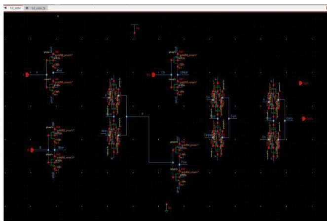
Fig.3 Transmission Gate Based Full Adder Design
