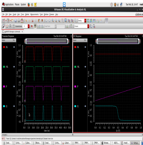
Fig.2. Transient and DC analysis of 6T SRAM Cell
