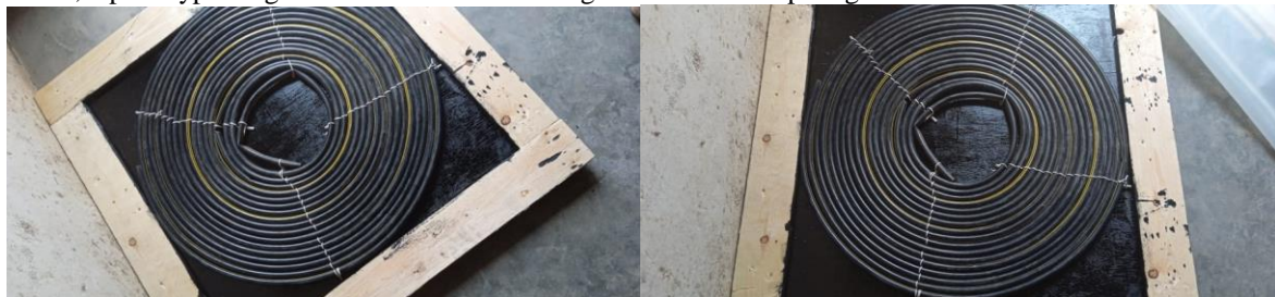
Figure 5 Based on research done, prototype of Longwave radiator made using drip irrigation hose
