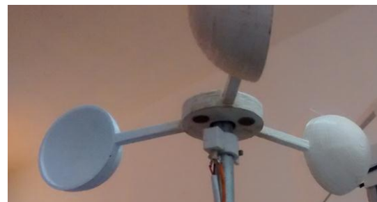
Fig. 4. Accommodation of the magnets, bearing and shaft of the mugs.
