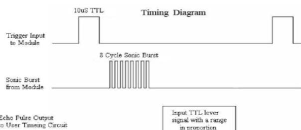
My model design plans to use 3 ultrasonic sensors for 270 degree field of view. All the three sensors work parlelly on the same principle the microcontroller triggers them using their respective pins, then calculates the time-based o echo signal length.[5][6]
