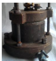
Figure 2: Final setup for testing permeability
