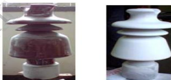
Figure 10. Pictures of non coated [left] and RTV coated [right] samples[4,11]
