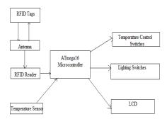
Fig 1. Main Block Diagram
