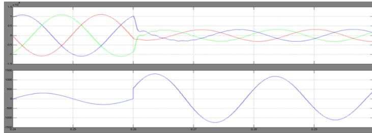
**Fig 10: Simulation result of wind farm fault current and voltages SFCL location in case of distribution grid (fault 1) feasible 1 location 1&4 with wind farm rating (2\*5=10MVA)**
