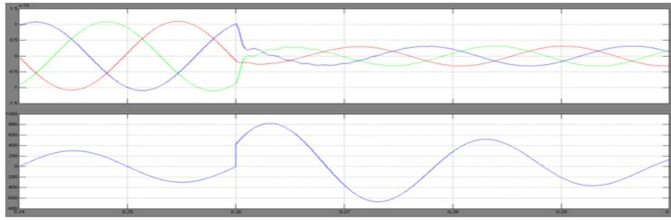
**Fig 9: Simulation result of wind farm fault current and voltages SFCL location in case of distribution grid (fault 1) feasible 1 location 3 with wind farm rating (2\*5=10MVA)**
