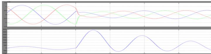
**Fig 13: Simulation result of wind farm fault current and voltages SFCL location in case of distribution grid (fault 1) feasible 1 location 3 with wind farm rating (6\*5)=30MVA**
