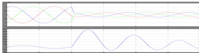
**Fig 8: Simulation result of wind farm fault current and voltages SFCL location in case of distribution grid (fault 1) feasible 1 location 2 with wind farm rating (2\*5=10MVA)**
