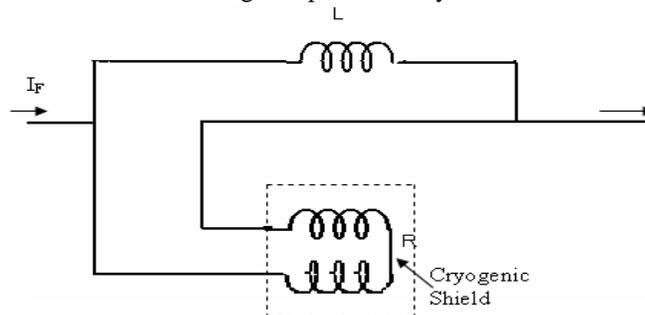
**Fig2: Superconductor FCL with inductive bypass element**
