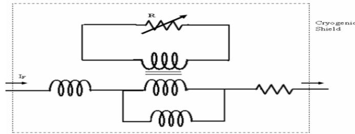
**Fig 3: Transformer coupled Superconductor FCL**
