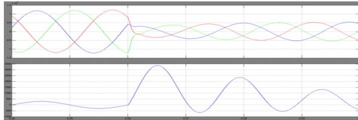
**Fig 12: Simulation result of wind farm fault current and voltages SFCL location in case of distribution grid (fault 1) feasible 1 location 2 with wind farm rating (6\*5)=30MVA**
