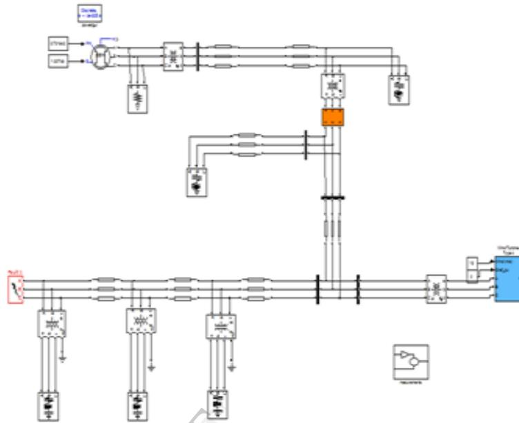
**Fig 6: Simulation Circuit Of A Grid Connected System With SFCL Location In Case Of Distribution Grid (Fault1)
