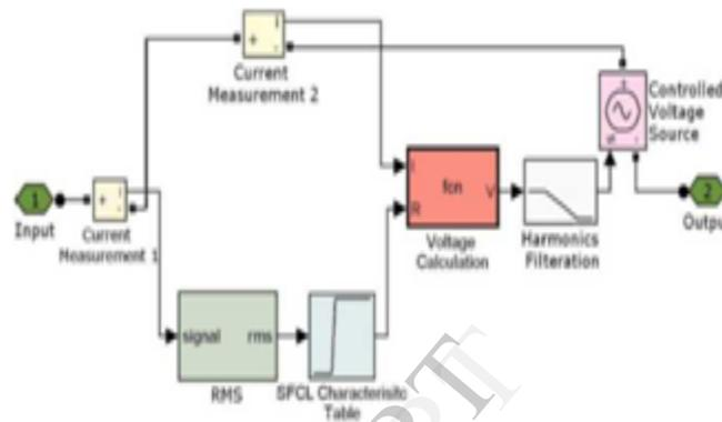
**Fig 5: Single phase SFCL model developed in simulink/sim power system**
