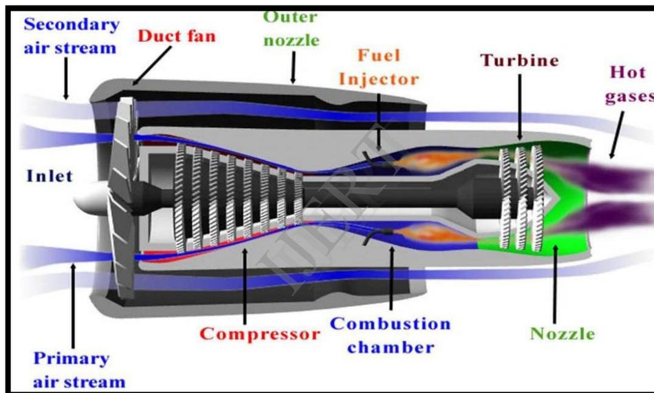
Fig 3: Turbofan Engines
