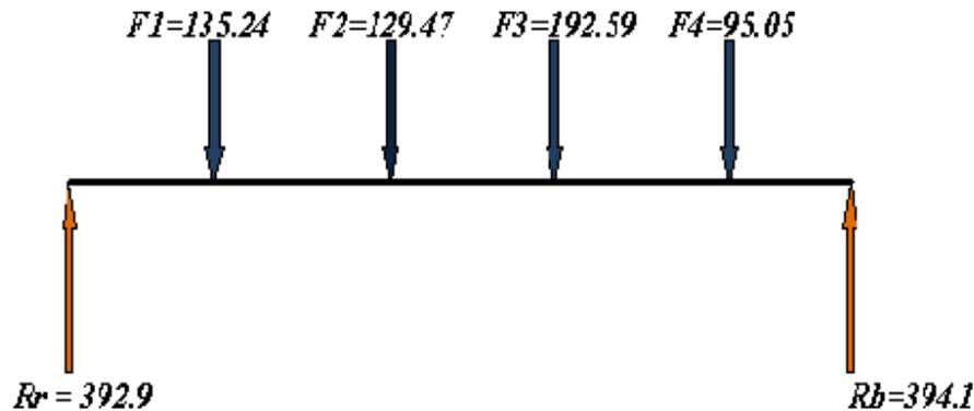
Total radial load acting on roller bearing  $F_{r_{roller}} = 3518.2 \text{ N} = 3.52 \text{ kN}$
