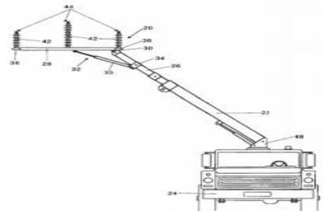
Fig. 6. Live line maintenance using ground based robots
