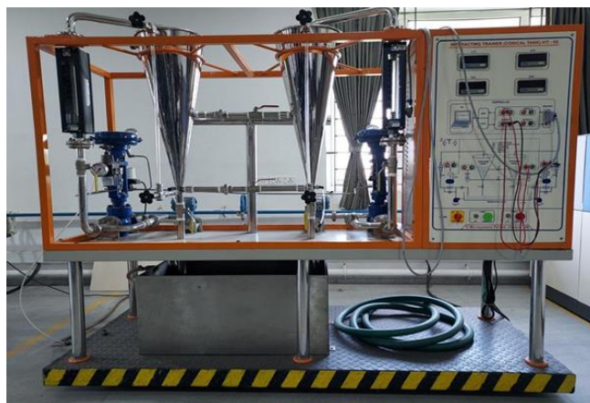
Fig. 1.1 Conical tank system
