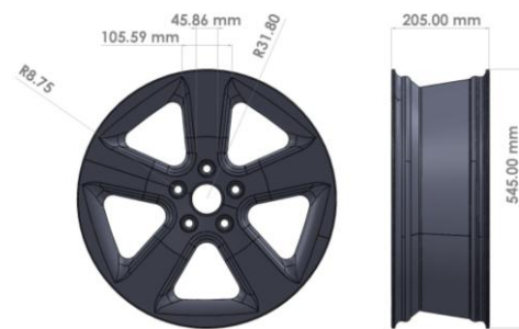
Fig 3. Design and dimensions (conventional rim)
