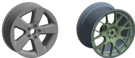
Figure 5. Finite-element mesh models of both rims
