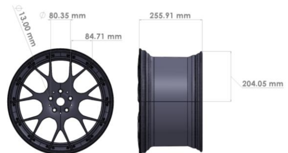
Fig 3. Design and dimensions (conventional rim)
