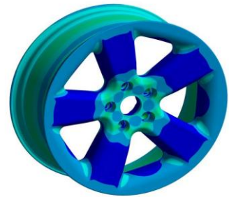
Fig 9. Conventional model — equivalent stress before TO
