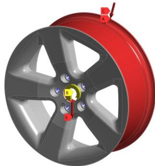
Fig 6. Boundary conditions of conventional design
