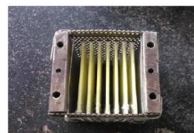
Fig.3: Special mould for the blocks
