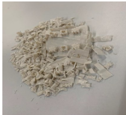
Figure 4: Infill from the printed lattice structure (Osadolor et. al., 2024)
