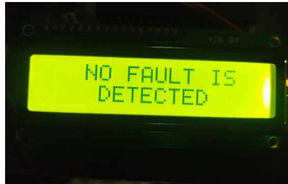
Fig (7). LCD under normal working condition,
