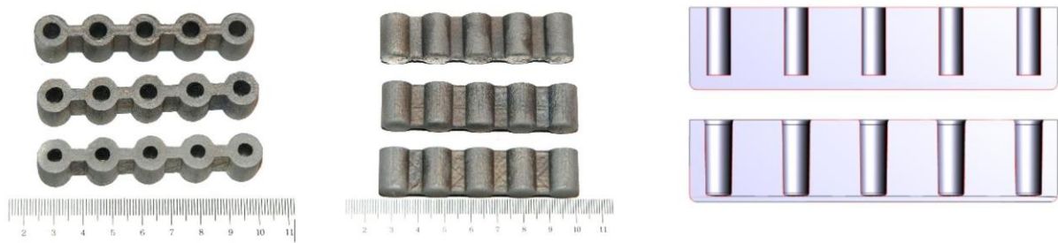
Figure 3: Specimens used to test ALtracs Plus screws
