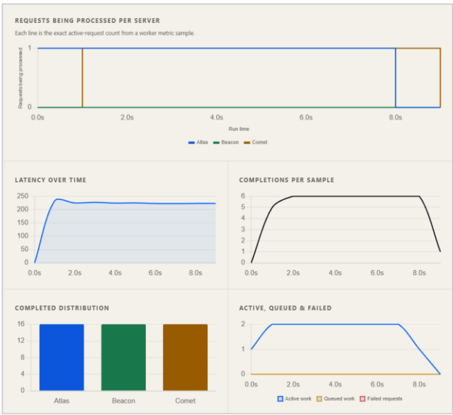
Fig. 7. Supporting time series for the steady-traffic run: requests being processed per server, latency over time, completions per sample, completed distribution, and active, queued, and failed work.
