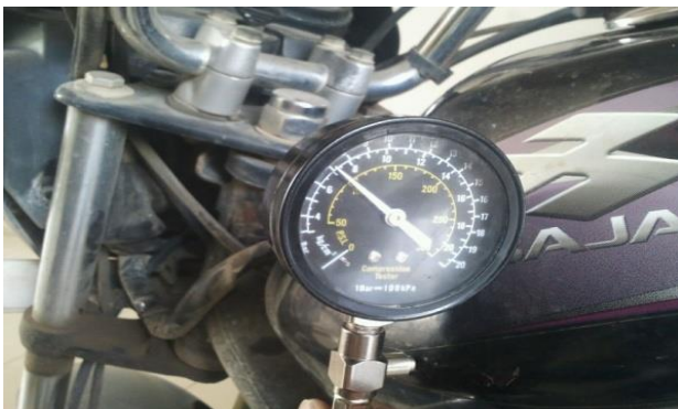
Figure 24: Compression pressure after Laser Surface Texturing
