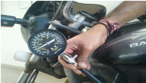
Figure 23: Compression pressure before Laser Surface Texturing
