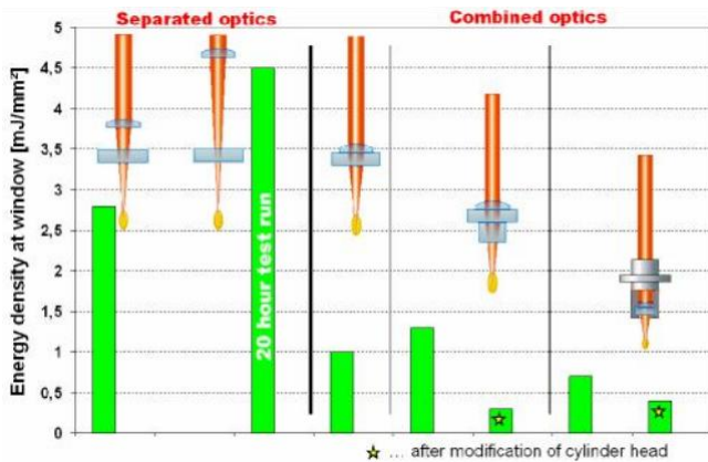
Fig. 10: Energy density at the window. It is higher for the separated optics. The higher the energy density, the better ablation works. The separated optics scheme should therefore be more reliable than the combined optics.
