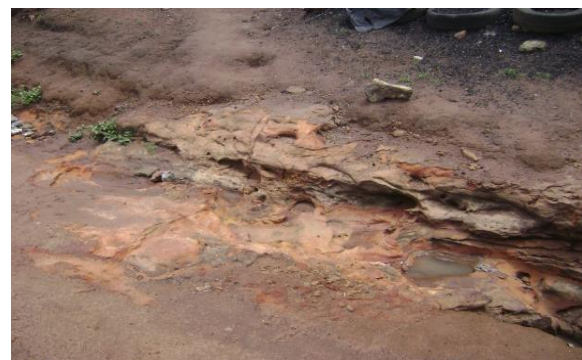
Plate 7A: An exposed impermeable layer in the Sumampa topsoil between 0-30cm depth.
