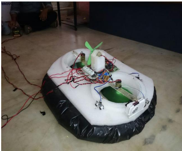
Fig. 6 The hovercraft after starting the hover motors
