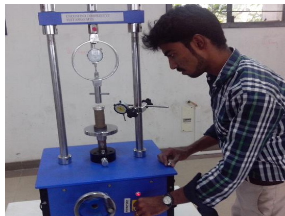
Figure 7.6: Unconfined compression Strength test set-up
