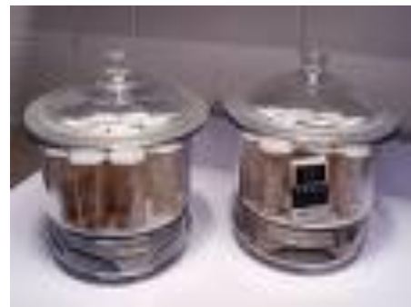
Fig 7.5: Curing of soil-cement Specimens in Desiccators
