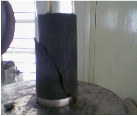
Fig 7.7: Failure Specimen @ higher water content higher cement content
