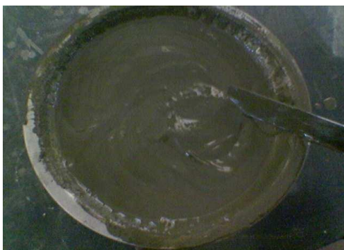
Fig7.2: Homogeneous clay-Cement with Cement slurry paste after mixing of w/c ratio = 0.6
