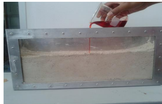
Figure 2. Releasing dyed LNAPL
