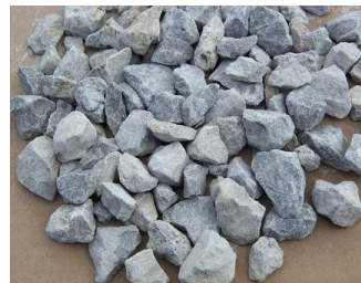
Fig1.1 AGGREGATES WITH NO FINES
