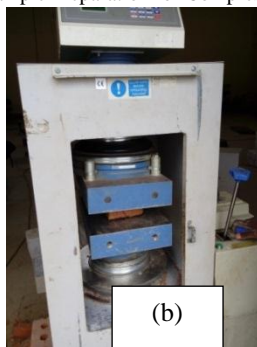
Fig 7. Testing Compression Test for Brick
