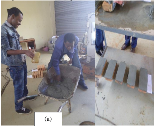
Fig 6. (a) Sample Preparation for compression test of Local Brick mortar capping (b) Sample Preparation for Compression Test
