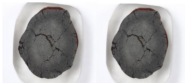
Figure 3 Picture of the cut etched sample reduced in 5 l/min H<sub>2</sub> for CVRD pellets
