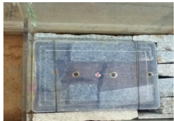
Fig. 4. Figure showing the points on depressed apron to which pressure transducers are fixed
