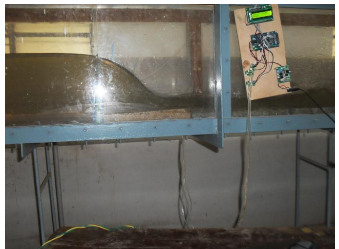
Fig. 11. Side View of the flume showing W-Jump for discharge No.8
