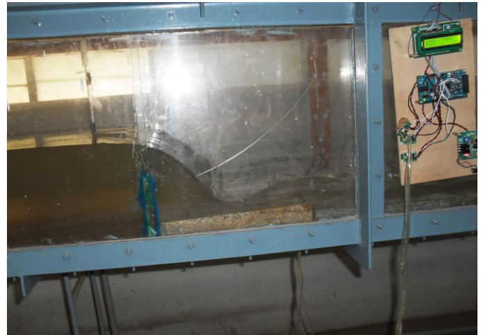
Fig. 9. Side View of the flume showing A-Jump for discharge No.4
