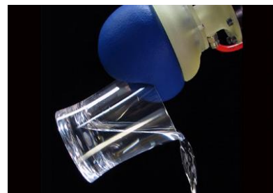
Picture 4: The robotic gripper conforms to the shape of the item it is lifting
