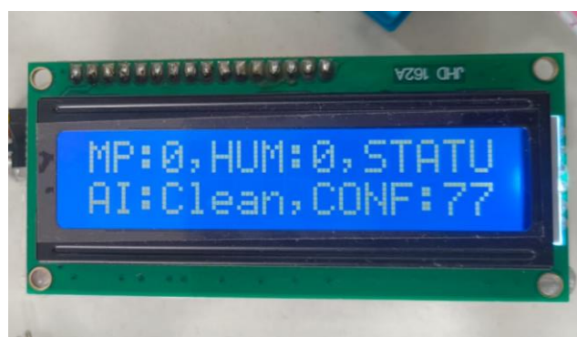
Fig. 4. LCD Display Showing Real-Time Water Quality Status and Environmental Parameters
