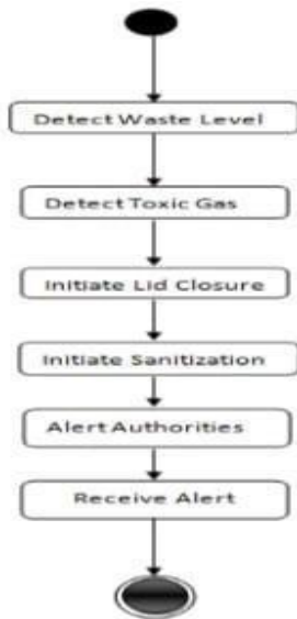
Fig. 2. Work flow of Waste Management System
