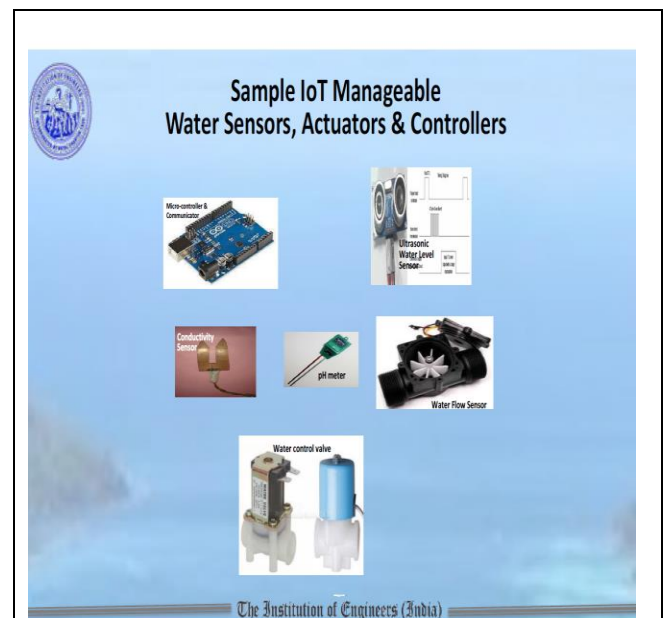
Figure 4. IoT manageable water sensors, actuators ,controllers
