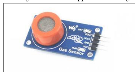
Fig-5: MQ-3 alcoholic sensor
